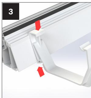
Locate the gutter bracket onto the external fascia and push down to locate the lower leg of the bracket. Assembly the outlets to the gutter profile ready for fitting. Ensure when fitting unions that the gutter is squeezed together to prevent dislodging the gasket
