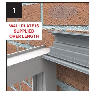
The wallplate is supplied over length and is designed to fit inside the sideframe. Therefore you can cut the wallplate to length or leave the wallplate at original length and (1) notch head of window frame or (2) notch bottom edge of aluminium wallplate to fit.
