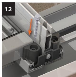
Ensure the glazing stop is pressed tightly up against the end profile. When in position use the fixings provided to fix the glazing stop down into the bar as shown.
