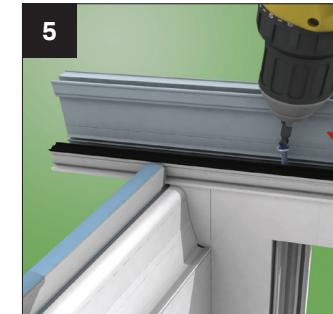
Screw fix the rafter down into the head of the raked frame at 500mm centres. Continue to fit the glazing as in steps 20-23 in main guide.
