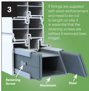
If firings are supplied with steel reinforcement and need to be cut to length on site, it is essential that the retaining screws are refitted if removed (see image)
