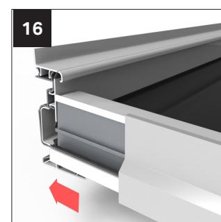
Apply silicone to the gable side capping and fit to the gable bars. These may require cutting in for a low pitch ridge.
