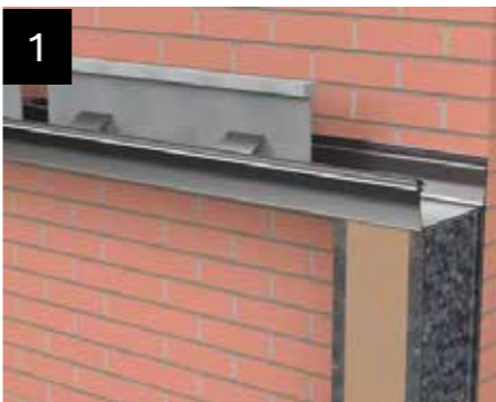
Lift the box gutter into position, taking into consideration the weight.
