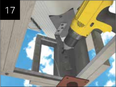
FIT THE STRAP CHA018 USING M4x13 SELF DRILL SCREWS, to the valley corner infill panel and the valley fixing bracket. It may be necessary to bend CHA008 to suit.
