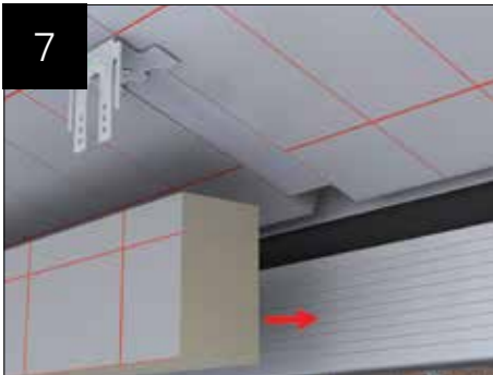
If the area around the box gutter is solid, additional insulation will be specified. Fit 90mm insulation block to front face of the internal box gutter fascia with sealant- this will help to prevent cold bridging.
