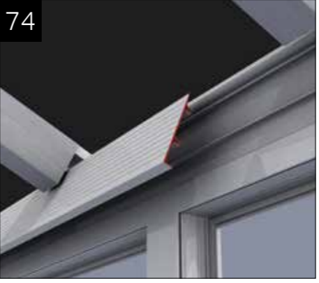
Attach fascia board to barbs built into the eaves beam.
