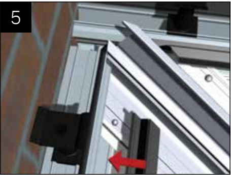
Re-fit the half ridge rain baffle. NOTE: If glazing with 24mm glass units or 25mm polycarbonate, the rain baffle upper leg needs to be set in the highest position.
