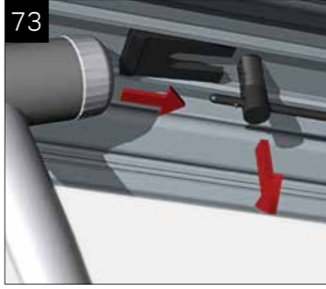
Pull down on the T bolt and tap the fixing wedge into place to secure the T bolt. Cut off the excess T bolt below the fixing wedge.
