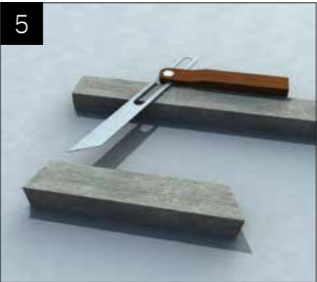
Transpose the angle onto the batten and create mitred cuts.
