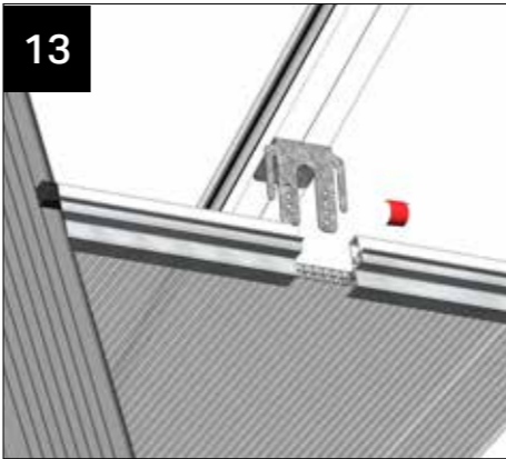
Attach the appropriate polycarbonate-LUVGS panels and fit as shown in the main internal insulated pelmet installation guide. (page 4).
