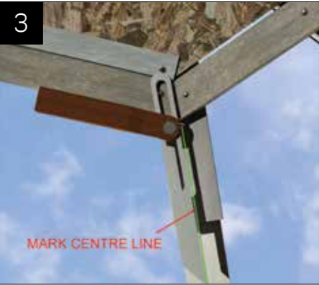
Use an angle finder to determine angle of each hip bar.
