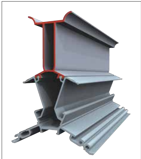
An aluminium bolster beam is factory stitched and extends along the entire length of the ridge and acts as one with the existing aluminium ridge body to virtually eliminate deflection.
