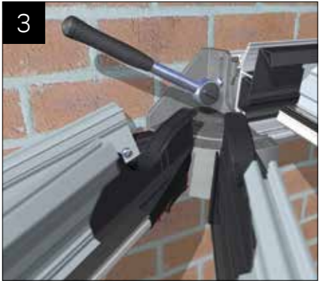
Check the half ridge for being level and then check the starter bar pitch. Drill and fix the die cast back plate to the host wall (avoiding mortar joints) using an anchor bolt suitable for the substrate. Drill and fix the starter bars(s).
