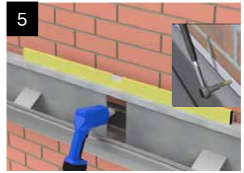
Ensuring the box gutter is level, fix back into the host wall through each gap in the I-beam and at both ends of the gutter using appropriate anchor fixings for the substrate. Dependant on access, a socket wrench may be used to reach behind the reinforcement.
