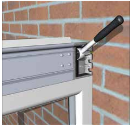
STRUCTURAL MOULDING EAVES/HOST WALL: Where the eaves beam sits against the host masonry wall, it has a structural moulding attached to the eaves beam. This has three fixing positions cast into it to allow attachment into masonry – choose the hole that directly lines up with solid masonry and attach using one resin anchor suitable for substrate / loads (other anchor types may be suitable).
