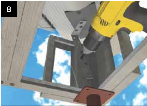
FIT THE STRAP CHA018 USING M4x13 SELF DRILL SCREWS, to the valley corner infill panel and the valley fixing plate. It may be necessary to bend CHA008 to suit.
