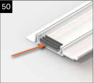
Fit the internal fascia claddings to the eaves beam, ensure the fascia corner packers are attached on the inside of the fascia at each corner.
