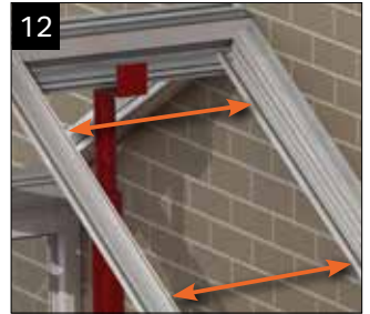
Check that the starter rafter and the first rafters are parallel. Ensure all bolts at both eaves and ridge are fully tightened.
