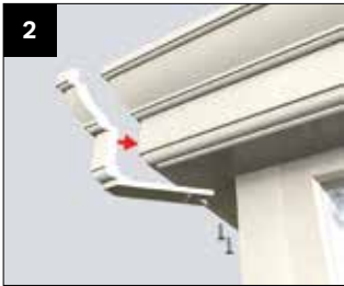
2 Whilst ensuring that the corner remains located in position, screw fix using self drilling screws CRN007
