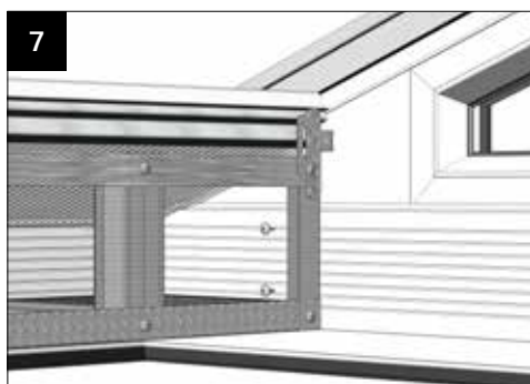
Fix the vertical frame into the fascia board using 2x CHAA006 (M4 x 13mm) self drill Phillips, wafer head screws (supplied).
