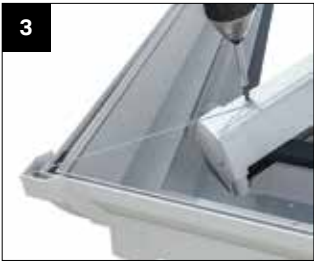
3 Finally secure the corner by screw fixing the wire tie to the glazing bar using self drilling screw CRN010
