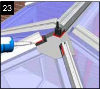
23 Once formed around the glazing, rafters and ridge, seal around these profiles.
