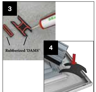
Take 'rubberized' sealer strips and generously butter with silicone. At 90° corner insert 'H' section and press down. Similarly apply at stop end or outlet positions.
