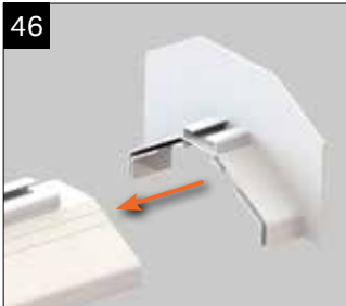
Now fit the ridge flashing trim to the ridge top cap, apply a bead of silicone inside to secure.
