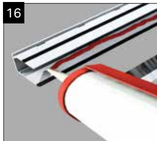
Take the glazing end profile and run continuous bead of sealant (appropriate for glazing) immediately behind the coextruded gasket (along the full length). Now seal the space between the glazing end profile and the sealed unit (see inset) at each end (DO NOT DO THIS ON POLY ROOFS).
