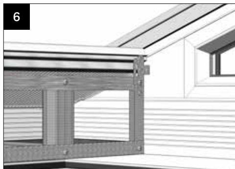
6 Fit the horizontal and vertical frames as shown in the main internal insulated pelmet installation guide. (pages 17 and 18).
