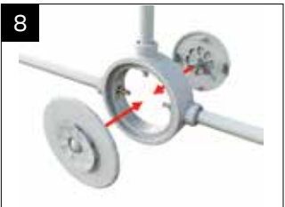
Offer up the two part rose cover, spin one half onto the threaded end of the other half.
