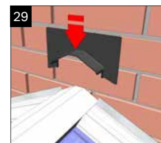
29 Lower wall flashing trim over ridge capping against the wall, pressing down and against the wall. Fold flashing over the trim or fit Conservafash into pre-cut slots in mortar lines following standard guide.
