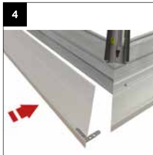
4 Fit the cleats (CRN001) to the desired side using the fixings provided (CRN006) as shown and assemble the remaining lower sections.
