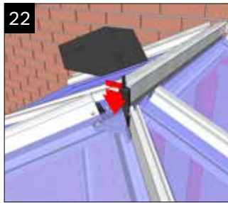
22 Fit glazing according to location plan. Fit weathering shield around sides of ridge and hip rafters. The shield is cut to allow the material to fold around the profiles.
