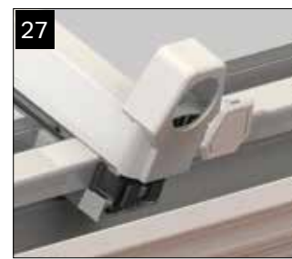
27 If you haven't fitted already, attach end cap fixing brackets. Fit the glazing bar end caps by sliding onto the end cap brackets. Push fit the insert into the end cap.
