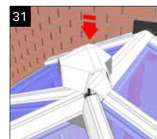
31 Fit ridge end cover locating on upstand on the Spider and over the hips, pressing down to seal.
