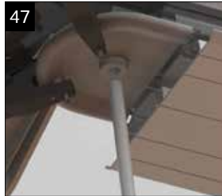
47 Insert the nylon threaded bar into the bottom of the spider.
