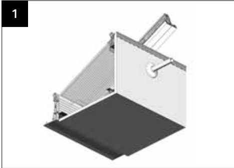
Once 12.5mm plasterboard is fitted, the tie bar rose (CHA005) flexes over the PVC conduit and should be spot bonded into position.
