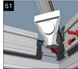
51 Fit the corner covers by trapping them behind the fascia sections. Insert the circular infill to finish.
