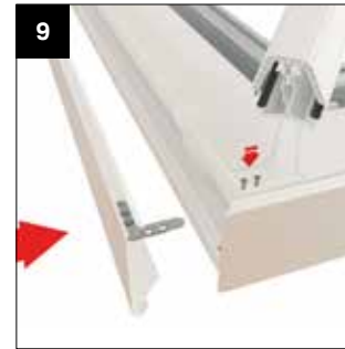
9 Fit cleats as shown in step 4. Offer up the next middle Cornice section. Secure corners using the cleats (CRN001) and fixings provided (CRN006).
