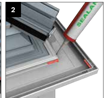
2 Silicone seal front and back edge of lower Cornice sections (be generous). Similarly butter 'DAM' sealer - position within 50mm of any stop end or outlet.
