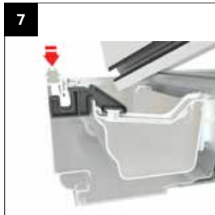
7 Take the middle cornice section and lower it into the lower cornice and support bracket.
