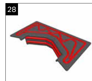
28 Liberally apply sealant to the back face and the underside of the ridge wall flashing trim.
