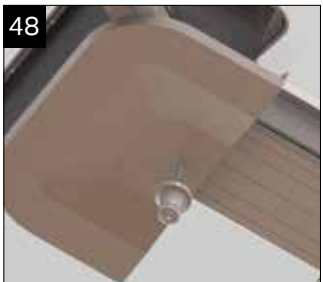
48 Offer up the internal radius end cap, use the threaded bar and the retaining boss to secure the internal cap in position. The threaded bar may require cutting to suit.
