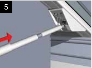
Offer up the horizontal pieces of PVCu conduit (large and small diameter).
