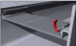
165mm box gutters These are supplied loose and MUST BE FITTED – they are a structural requirement of the roof. The straps must be installed within 75mm of glazing bar centres (when measured from centre of the strap to the centre of the bar). To install these straps, simply 'nip up' as shown.
