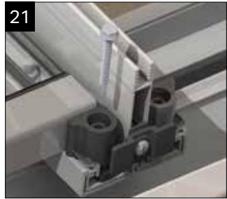
21 Ensure the glazing stop is pressed tightly up against the end profile. When in position use the fixings provided to fix the glazing stop down into the bar as shown. Ensure clip offers maximum support to glazing at all times.
