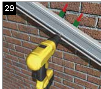
Drill the starter bars/masonry within 200mm of the ridge and eaves beam plus at least one more equidistant between the two. Pack out to support the starter bar behind each fixing before fitting the correct masonry anchor.
