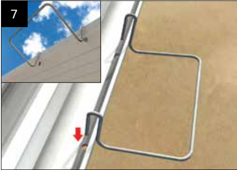
Refit the clips with the clip leg extending through the holes.
