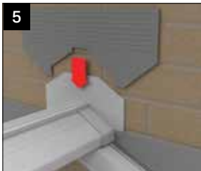
Having added last stepped flashings each side of the ridge 'Butter' the reverse side of the saddle trim and place over the ridge body.
