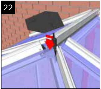
22 Fit glazing according to location plan. Fit weathering shield around sides of ridge and hip rafters. The shield is cut to allow the material to fold around the profiles.
