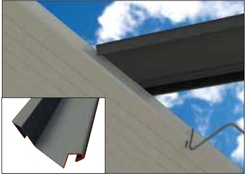
In valley situations the closure trim sits onto the valley drip profile. The nose of the closure trim must be notched as shown above, this allows the trim to sit flat.
