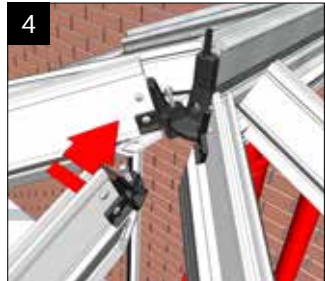
If specified, fix central rafter using the same method as the hips by pushing the Spider arm hook over the Spider.
