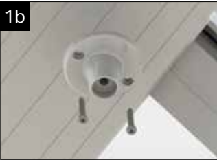
Tie bar at ridge Mark the position of the where the tie bar meets the ridge, fix the ridge fixing cover using the self tapping screws provided.
