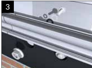
Drill 6.5mm holes through the box gutter and sleeve (at positions shown, ensuring both halves of the box gutter are flush together) and fix using the bolts, nuts and washers provided and in the order shown. Trim any excess off the bolt head before fitting the internal cladding as it may foul.
