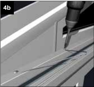
4b Fix wire ties at an angle as shown, ensure the gutter cover is parallel to the frames/roof line.
