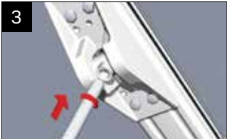
Measure, cut and attach the horizontal threaded bars (ensure sufficient engagement of the bar into the brackets) – it is essential that the tie bar boss is central. Take the boss ring, and loosely assemble the threaded bars to check they terminate inside the ring. Dis-assemble.
