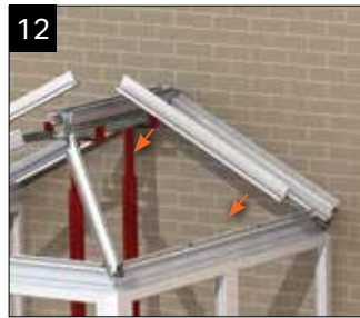
Continue to support the ridge and offer up the rafters that meet the ridge. Locate onto the double bolts at the ridge and bolts at the eaves.
