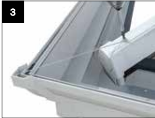
Finally secure the corner by screw fixing the wire tie to the glazing bar using self drilling screw CRN010
