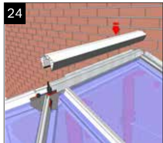
24 Fit ridge capping by locating barbs in ridge profile and knocking down along its length. Use a timber drift and dead-blow hammer to avoid damaging the capping.
