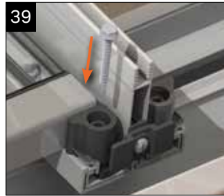
Ensure the glazing stop is pressed tightly up against the end profile. When in position use the fixings provided to fix the glazing stop down into the bar as shown. Ensure clip offers maximum support to glazing at all times.
