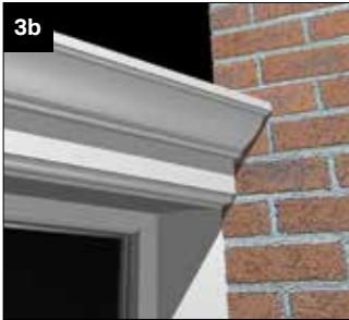
3b GUTTER COVER & GABLE EAVES BEAM DETAIL - Used on lean-to styles with raked frames or duo-pitch gables that use the gable support beam. Fix lower section as shown - continue with the remainder
