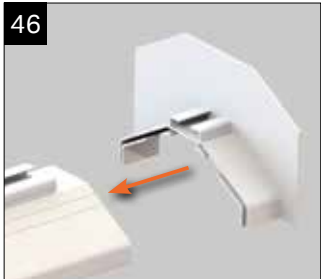
Now fit the ridge flashing trim to the ridge top cap, apply a bead of silicone inside to secure.
