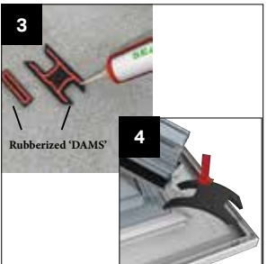
Take 'rubberized' sealer strips and generously butter with silicone. At 90° corner insert 'H' section and press down. Similarly apply at stop end or outlet positions.
