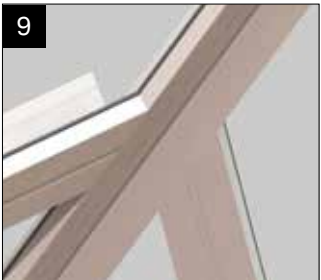
Once fixed, minor adjustment maybe required to align the under cladding flush with the under side of the hip, this can be done by adjusting the bolts to suit. Repeat these steps until all jack rafters are fitted. Fully secure all rafters and hips.
