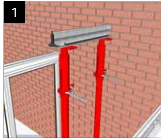
Support the ridge against the host wall centrally between the frames. Ensure supported throughout the assembly process until all components are fully secured.
