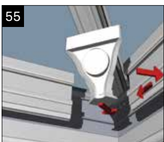
Fit the corner covers by trapping them behind the fascia sections. Insert the circular infill to finish.
