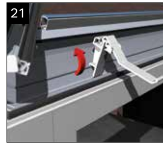
Fit all the gutter brackets supplied with the kit at maximum 750mm centres and maximum 200mm from each corner.
