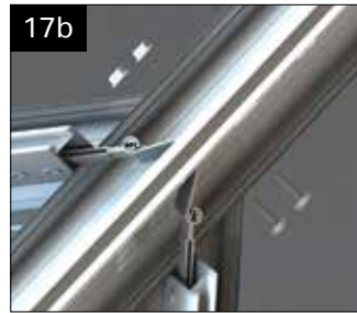
If two jack rafters are aligned either side of the hip, a M6 x 25mm bolt is required to fix both sets of brackets through either side.
