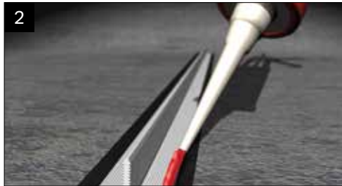
Now take the upper section and lay it face down onto a smooth clean surface. Using the relevant sealant (MS Polymer sealant such as Rotabond 2000 must be used on self cleaning glass), apply a generous bead to each side, immediately behind the gasket.
