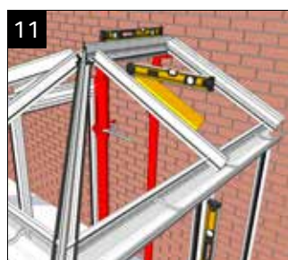
Check rafter centres are square and that the ridge is level. Check side pitches and that side frames are plumb.
