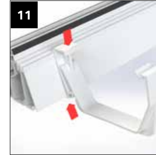
Locate the gutter brackets, stop end and stop end outlet and lift into position on the external fascia. Push down to locate the lower leg of the bracket. Assemble the rain water pipe, attach to the gutter and screw to the frame.
