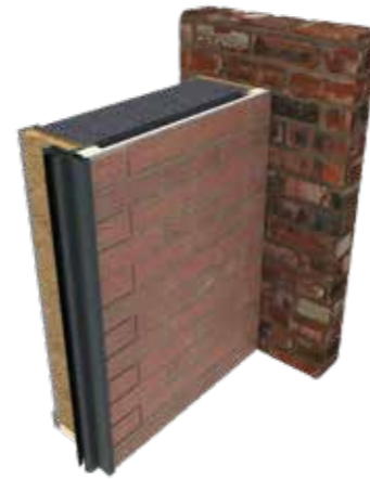
Render / brick abutments wall 665mm or 3 bricks.
