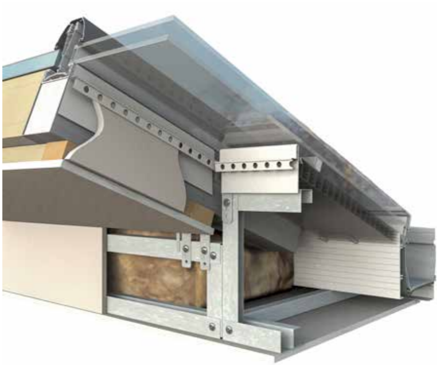
Box Gutter - solid/glass - below fascia
