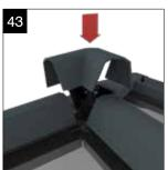
Fit the ridge end external cover and press down firmly clipping in place.
