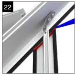
Seal the area where the hip rafter abuts the jack rafter as shown above
