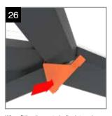
When fitting the central rafter internal cover on the aluminium internal lantern. The front leg is inserted between the aluminium cladding and PVC cladding on the central rafter. The cover is then pushed into place around the ridge cladding.
