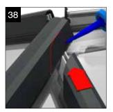
If the project contains jack rafters, apply MS polymer to the hip top cap where the jack rafter cap will abut. Push the rafter cap up against the hip and point any visible sealant that seeps out.
