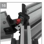
If the project contains central rafters If the project contains central rafters between the hips. Tighten the central between the hips. Position the rafter rafter bracket screw to ensure it is properly between the two hip rafters, secure secured.
