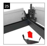
If installing an aluminium internal lantern. Prior to glazing the lantern, fit the internal ridge end covers. These clip into place locating around the ridge cladding, with the front leg locating over the hip claddings.
