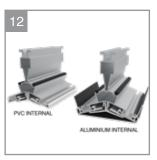
Ensure the ridge claddings are fit to the ridge body prior to continuing with installation. The PVC internal claddings are comprised of three PVC extrusions that slide onto the aluminium ridge body. If aluminium internals are specified this should be slid over the PVC claddings.
