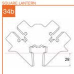
Cut the ends off two weathering shields. Ensure glass is clean and dry before fitting. Peel back protective film from shields and position (adhesive face down) on glass, locating around the ridgeLOCK and hip rafters.
