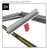
If the project contains side rafters: Locate the rafter on the bolts at the ridge and eaves, once in position secure with flanged nuts. Check the ridge is level.
