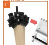
Ensure the assembled ridgeLOCK is propped throughout the assembly process. Fit each hip rafter to the tenons of the ridgeLOCK. Secure in place into pre drilled holes using M5 x 16mm screw in the upper hole and the M5 x 20mm screw in the lower hole
