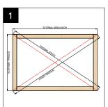
Construct the up-stand to the flat roof with a minimum of 150mm tall kerb (minimum of 70mm wide). Check that kerb is square by measuring diagonals. Ensure the kerb is built to external kerb dimensions that match that specified for the lantern.
