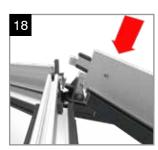
If the lantern is specified with a central bar and aluminium internal claddings. The hip rafter will have a notch applied to the cladding removing 52mm where the central rafter intersects the hip rafter. Once fitted the central rafter and the PVC rafter cladding will extend beyond the aluminium cladding of the hips while the central rafter aluminium cladding will terminate into the sides of the hip aluminium claddings.
