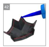
Apply a small bead of MS polymer to the inside of the external cover (as shown) around where the part meets the glazing rafter top caps and the ridge top cap. If fitting a square lantern, see step 44.
