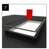
Position the assembled eaves beam frame on top of the kerb, centre this eaves frame over the opening ensuring it is square (check diagonals). Fix down to the kerb using appropriate fixings not supplied.
