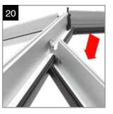
If aluminium internals have been specified on a lantern with a jack rafter. The aluminium cladding on the rafter will finish flush with the top end of the bar. The rafter will then terminate into the side of the aluminium cladding on the hip bar
