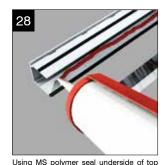
osing wis polymer sear understoed to deface of glazing end profile as shown. Depending on the roof specification this can either be a PVCu or Aluminium profile. The end profile is to be aligned flush with the glazing in transom locations, it will then stop short of the glass by 5mm at hip
