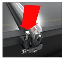
Push the glass stops up to meet the glass end profile, ensure that the lower edge of the glazing is running parallel to the kerb. Then using fixings provided secure the glass stops in place.
