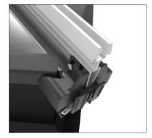
Ensure the glass units are pushed up towards the ridge and that the glazing is securely located behind the glassLOCKs at the hips.
