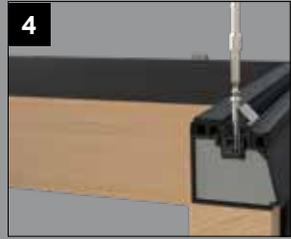
Firstly check that all aluminium spacer sleeves are in place in the fixing holes. Ensure you use all the clips provided. Position clips (FRICB001M) into location holes and fix using the provided (FRFC008-100) 100mm long screw.
