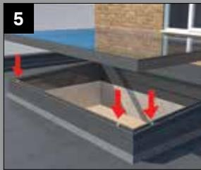
Fit the top glass frame onto the PVCu frame. Carefully lower into position and then apply downwards pressure to opposite sides to activate clips (You will hear a click).
