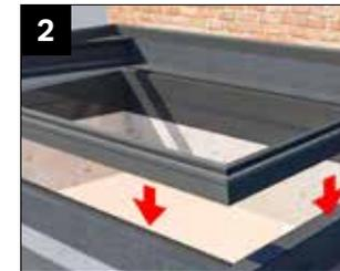
Position PVCu welded base frame and align with internal kerb face.
