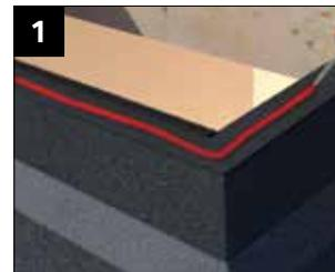
Apply a generous, continuous bead of silicone to the top surface of the kerb as shown.
