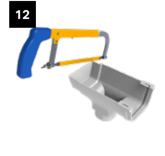
If a stop end outlet is to be used in an inline outlet situation, use a hacksaw to remove the stop end as shown. A stop end outlet is used for inline situations when the inline variant is not available in the specified colour.
