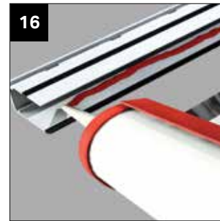
Take the glazing end profile and run continuous bead of sealant (appropriate for glazing) immediately behind the co-extruded gasket (along the full length). Now seal the space between the glazing end profile and the sealed unit (see inset) at each end (DO NOT DO THIS ON POLY ROOFS).
